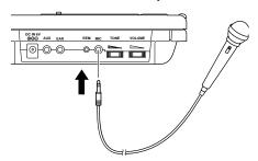
**Note:** If the external microphone has a separate, smaller plug for remote operation, insert that plug into the **REM** jack. Then you can use the microphone's remote switch to stop or start recording.
